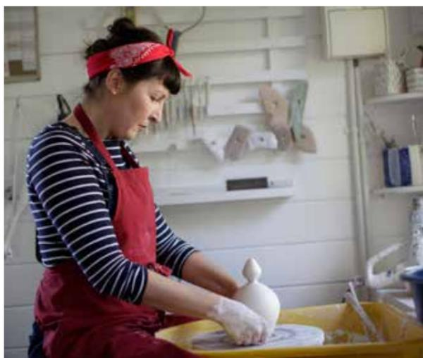
**7** I cut the pot off in one swift movement using a wire or fishing line. If you stop or slow down while doing this you can get lines on the base that may lead to cracks.
