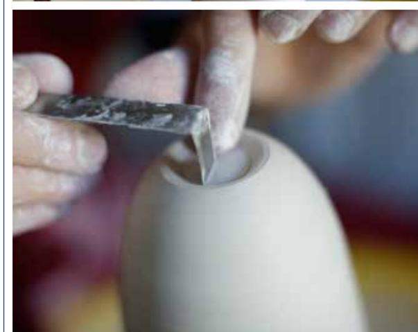
**10** I use both European and Asian-style turning tools alongside a couple that I handmade myself from metal binding and string, which I love. I work on the base curve to create a foot ring, which I think helps lift any shape.
