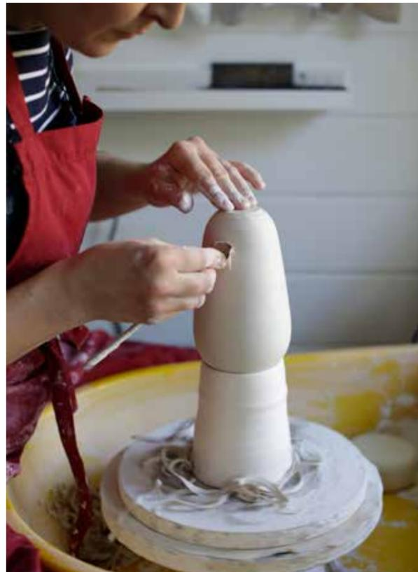
**9** I place the pot upside down into one of my chucks – a dry cylinder with a heavy base – to secure it in place while I turn and trim it. I have a selection of chucks in different diameters to fit pots in a range of shapes and sizes. As the chuck is only dried and not fired I can fix it to the wheel temporarily by simply moistening the base. Turning each piece is a key part of my making process – I want each piece to be pleasing no matter which way you see it.
