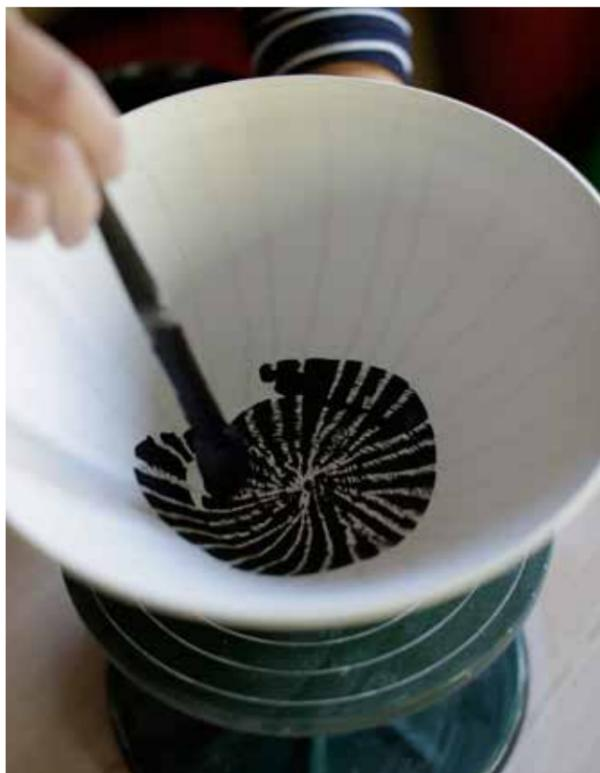
**14** I then glaze the pot – the pastel lines repel the glaze fluid. I spray some of my glazes, others I dip, some I need to brush on – it depends on the ingredients of the glaze I've mixed together and how they disperse in the liquid. It takes time to get to know a glaze and how it behaves in application, on your clay and in the kiln with your chosen temperature. I fire between 1260-1275°C, depending on the glaze that I'm using. I fire mostly in an electric or a gas kiln.
