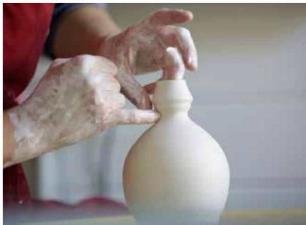
**4** Once the belly is complete, I start the top part. It is important you know what shape you want to achieve before you start. I slow down the wheel at this point and work bit by bit to narrow the neck then form the top into a conical shape. (There is a different shape shown in the accompanying video – the double bauble, shown in step 8).
