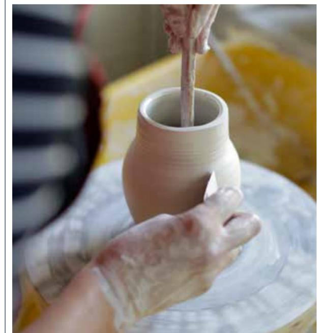
3 I then shape the belly using a throwing stick. This allows me to keep the vase's opening narrower than if I was using my fingers.
