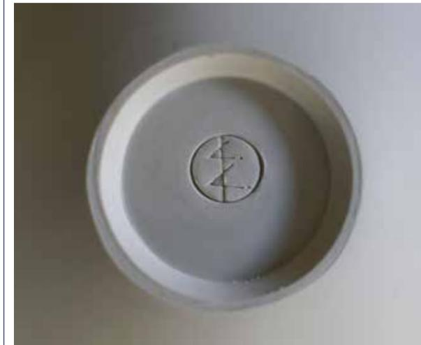
**11** As the final step, I press my makers mark stamp into the base of each piece. After a week of drying, the pots go into the bisque kiln at 950°C.
