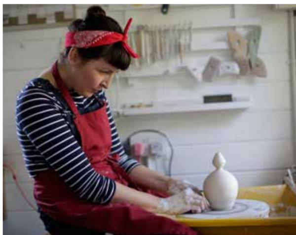
**6** I use an old store card to smooth the surface of the whole pot and tidy up the foot by scraping away any excess clay, holding the card at an angle.
